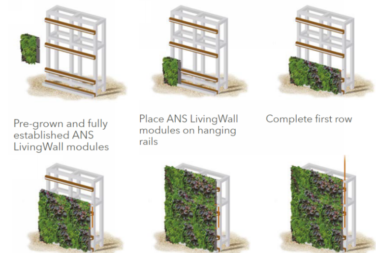
Pre-grown and fully established ANS LivingWall modules Place ANS LivingWall modules on hanging rails Complete first row Install irrigation pipe on each row of modules Build the living wall up layer by layer. Each module is planted to give desired effect. Finished wall connected to irrigation system.
